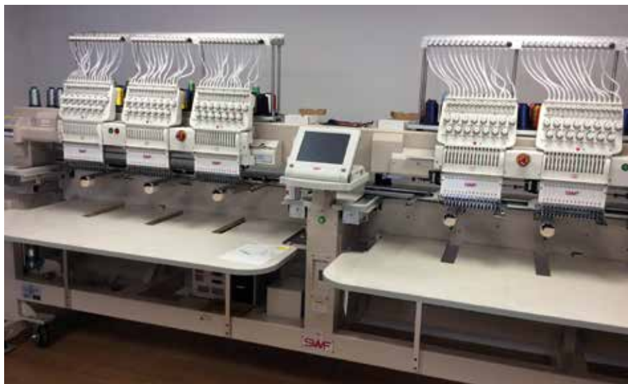
The 6 head embroidery machine purchased as part of this project
