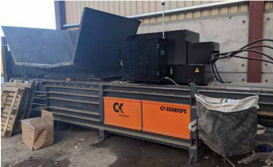
The horizontal baler installed at William Brown's new recycling centre near Donaghadee
