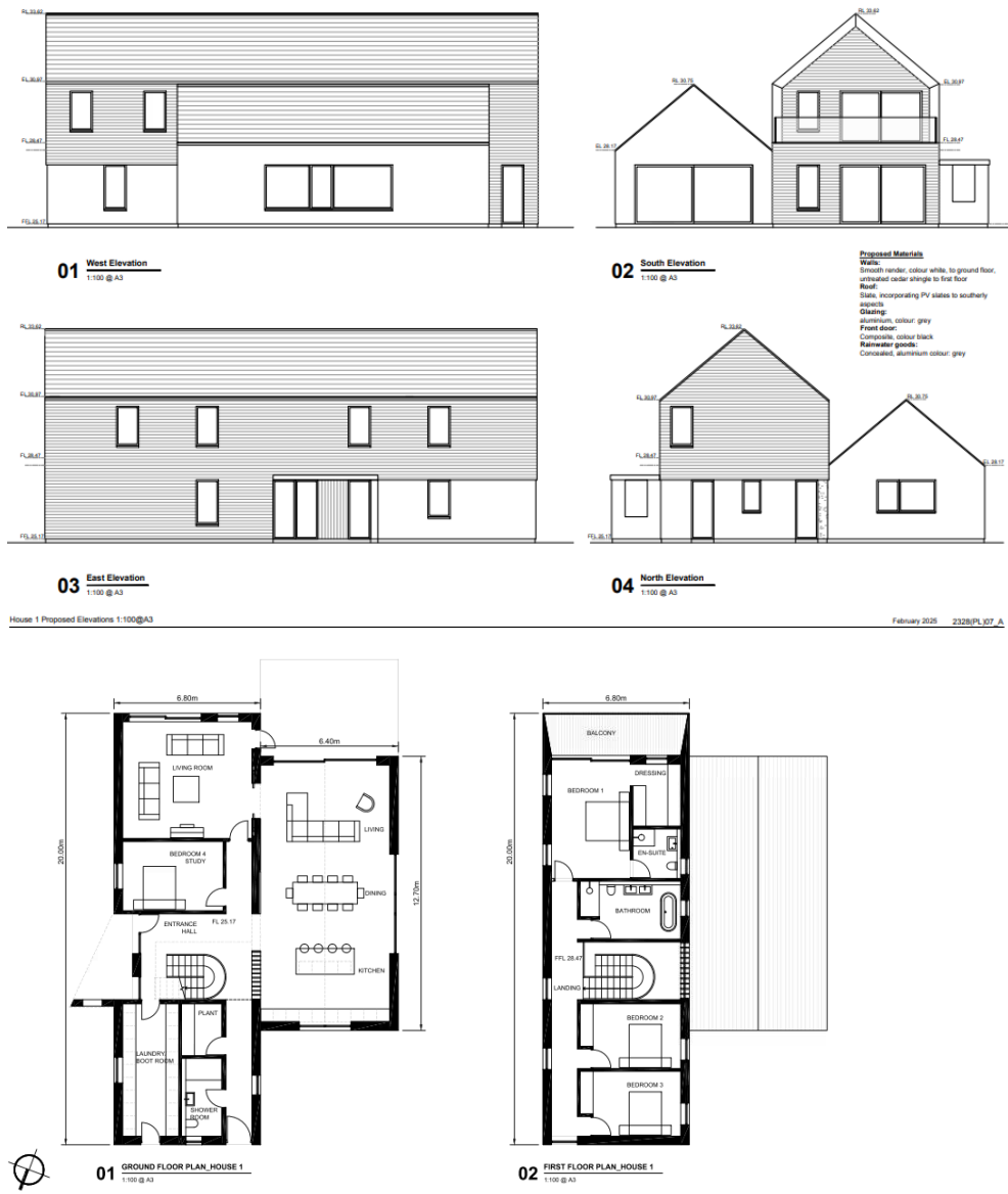
Fig 8: House type 1 elevations and floor plans
