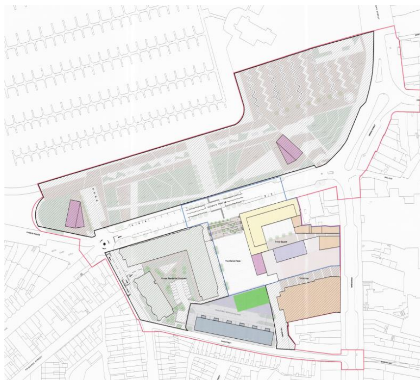
Figure 8 - Phase 3 (Approved) – Commencement of work on hotel, kids' zone, offices, Market Square and associated steps and completion of works to Trinity Square, installation of raised table at Queen's Parade, marking of loading bays at eastern end of Queen's Parade marked out.
