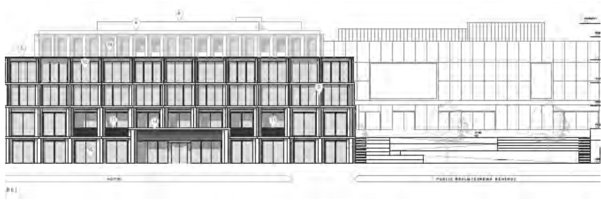
Figure 46 – Original proposed Queen’s Parade elevation showing roof plant on hotel and cinema buildings prior to amendments
