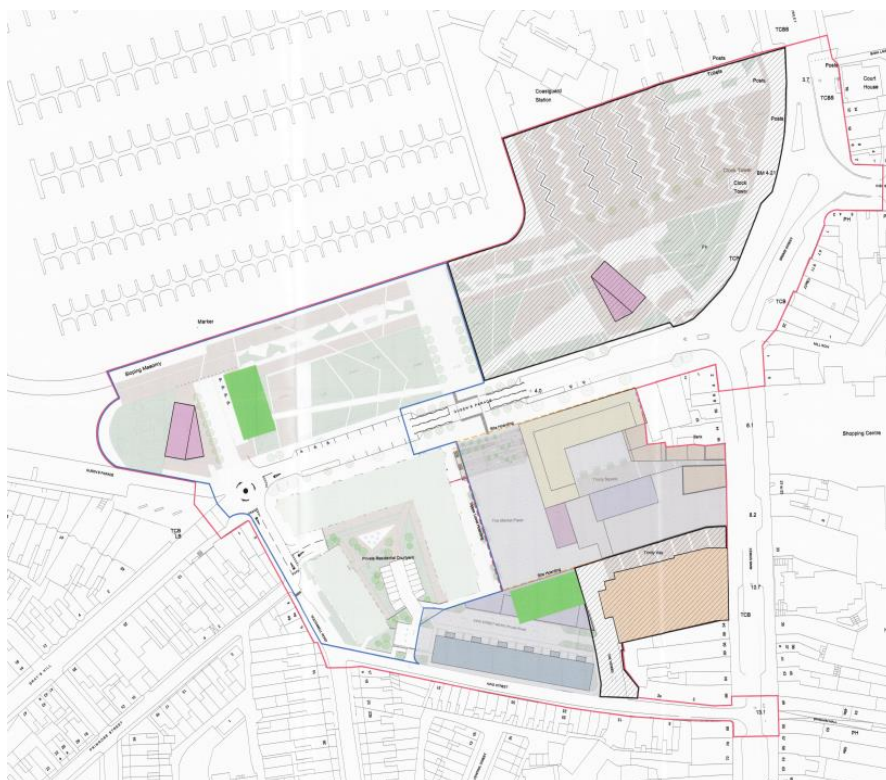
Figure 6 - Phase 2 (Approved) – Delivery of remaining public realm at Marine Gardens and commencement of development on under-croft car park and residential blocks 1 and 2 with all remaining buildings demolished with exception of King Street, widening of Southwell Road, marking of loading bays at western end of Queen's Parade
