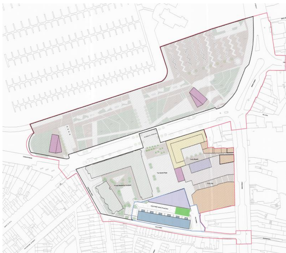
Figure 10 - Phase 4 (Approved) – Demolition of King Street terrace and completion of 24 new residential units and cinema building and completion of all hard and landscaped surfaces.
