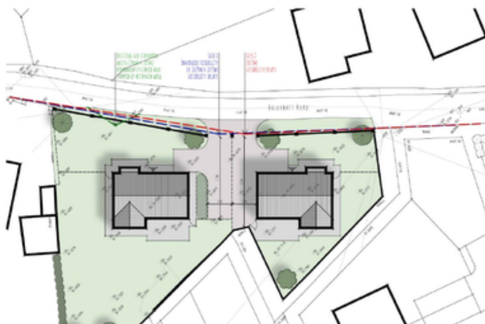
Figure 8: Plan showing existing access permanently closed off and proposed access to sites 1 and 2.
