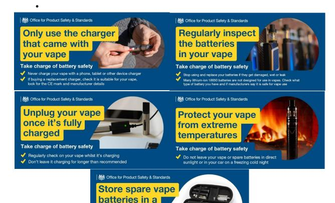
Keep batteries away from other metal objects like coins or keys in a pocket or bag to avoid accidental contact as this can cause a short circuit
